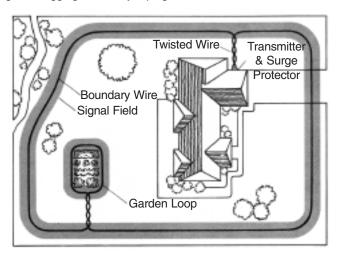
**Boundary Wire:** The boundary wire carries the coded radio signal around the perimeter of your property. It is rated for underground burial.
