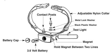
**Adjustable Collar**: Both the R7 and R8 receivers come fitted to an adjustable nylon collar. The collar should be positioned above the dog's regular collar. The collar should be adjusted to insure that the contact posts touch the skin on the dog's neck. *Check the fit for the first few days of wear to insure that the collar is not too tight or causing irritation to your pet's neck.*
